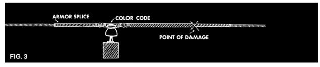
The *Armor Splice* combines the features of both *Armor Rods* and *Conductor Splices*, which are described in their respective catalog sections. The *Armor Splice* should be considered when damage occurs in the "support area," or where installation would locate the ends of repair rods within 6 inches of existing rods.
